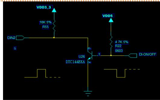
DO: Digital output DO, can be used to control external drive devices, such as relay switches
